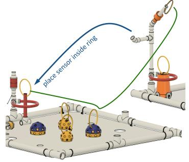
Temperature Sensor Connector Placement Option A (solid) – Option B (dashed)
