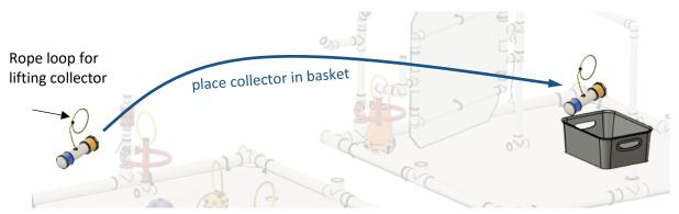
Water Sample Collector Closure and Placement
