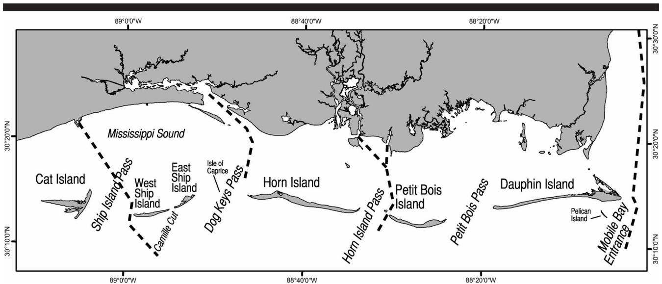
Figure 1. Locations of the Mississippi-Alabama barrier islands and associated tidal inlets. Deep-draft shipping channels (heavy dashed lines) leading to the mainland are maintained by periodic dredging.
