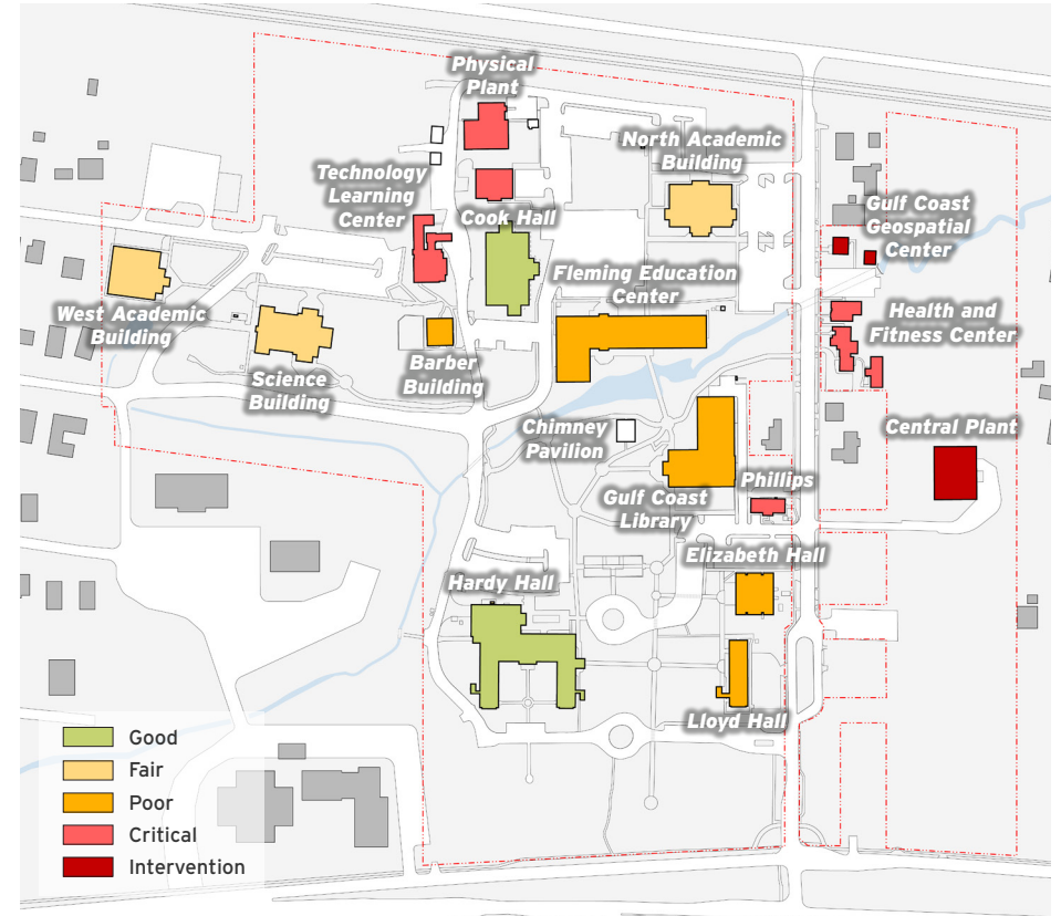
Projected ten-year facility condition index (FCI)
